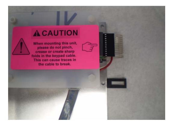
2. When mounting the MCS-Keypad be sure to fold over the black ground tab on the right side of the keypad and then fasten the screw on the keypad.
